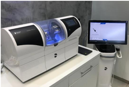
Figura 15 – CAD/CAM Dentsply Sirona (scanner e fresadora).
