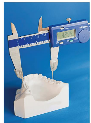
Figure 4 - Intermolar width measured on a dental cast by means of a digital caliper.
